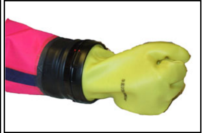
21. Hold the lock ring to the glove with your hand. Clench your fist inside the glove and turn the glove outwards, until the red and yellow dots are next to each other. The lock rings will now be hooked on.
