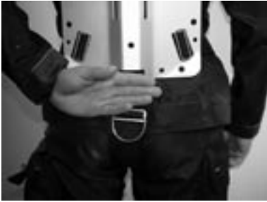
Fig. 7: Rear D-ring placement
